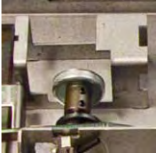
Plexus friction plate removed ready to receive the remote motor
